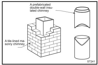
Fig. 2 Standard chimney types.
